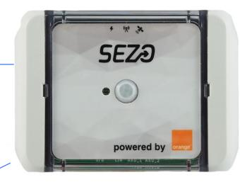
battery-powered (3.6V 8000mAh), wireless charging in Qi standard
